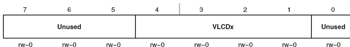
LCDVACTL1, LCD_A Voltage Control Register 1
