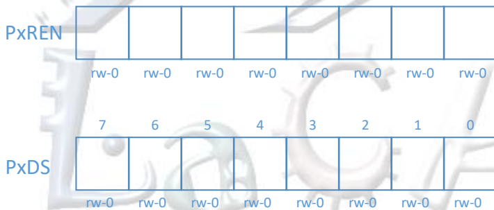
Figure 4. Programmer's view of PxREN and PxDS registers.
