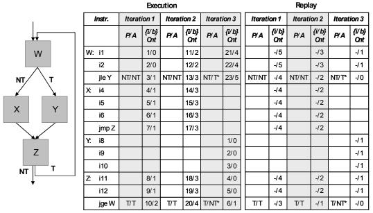
Figure 4. Tracing and replaying the sample execution.
