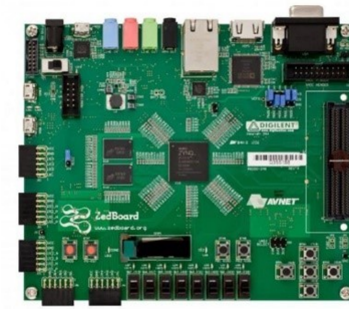
Figure 7.1 Zedboard Development Board [29]
