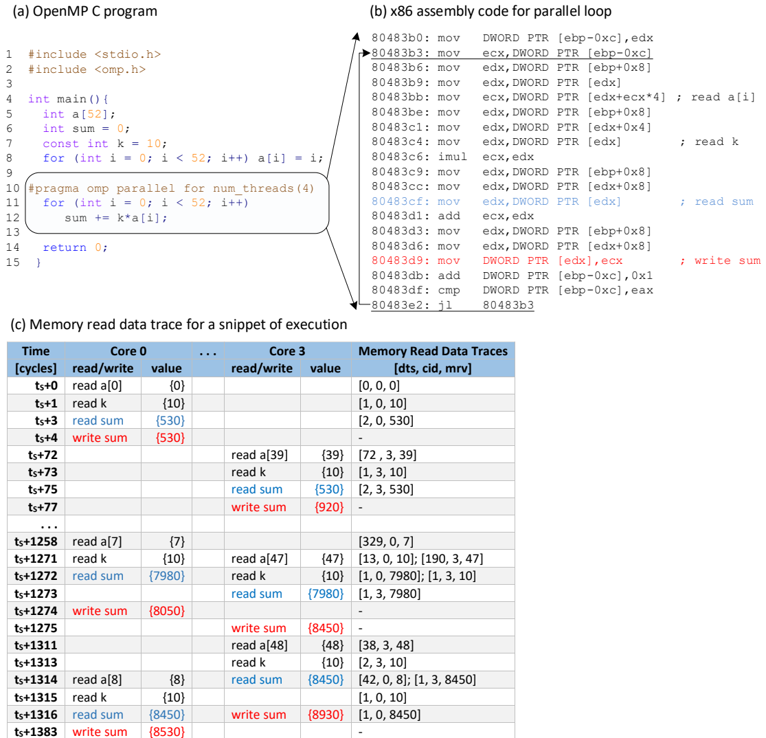
Figure 2.2 Memory Read Data Value Tracing Example
