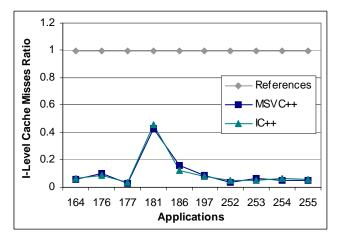
Figure 5.8 Comparison of I-level Cache Load Misses
