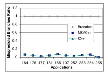
Figure 5.6 Comparison of Mispredicted Branches Retired
