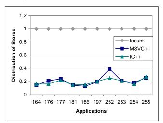
Figure 5.4 Comparison of Stores Retired
