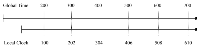
Figure 1. To synchronize to global time, a node must compute the offset between its local clock and the global time as well as the skew or rate at which its clock is drifting slower or faster than global time. The numbers shown are merely illustrative.
